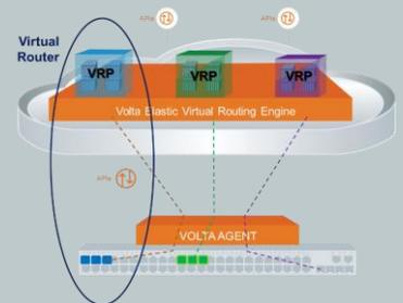
*The vAgent works in tandem with a VRP to create Virtual Routers. Up to 255 VRs can be supported on a single device.*
