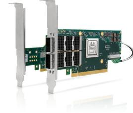
1. By default, the above products are shipped with a tall bracket mounted; a short bracket is included as an accessory.
